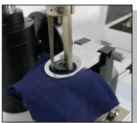
Clamp go down until reached surface of test fabric, rotate thread disc tapered end, button be clamped.
